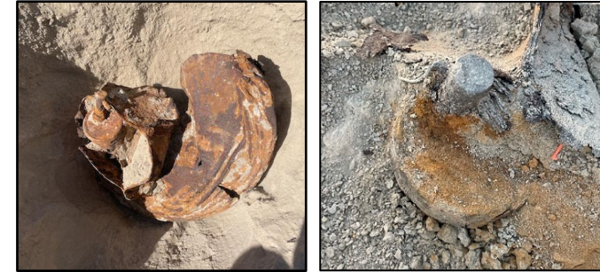
Remnants of a M38A2 100-lb sand-filled practice bomb and 3-lb black powder spotting charge
